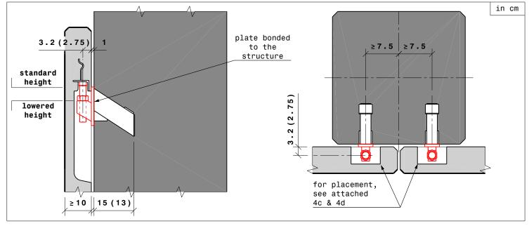
N.B.: - between parenthesis you will find the values for Hercules Snella 15 and 25; - all the brackets are designed to support only vertical charges, so, horizontal actions cannot be applied.
