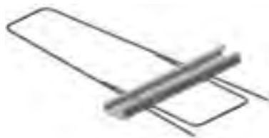
ANCHORAGE PROFILE B.S.s. with bracketing rebars
